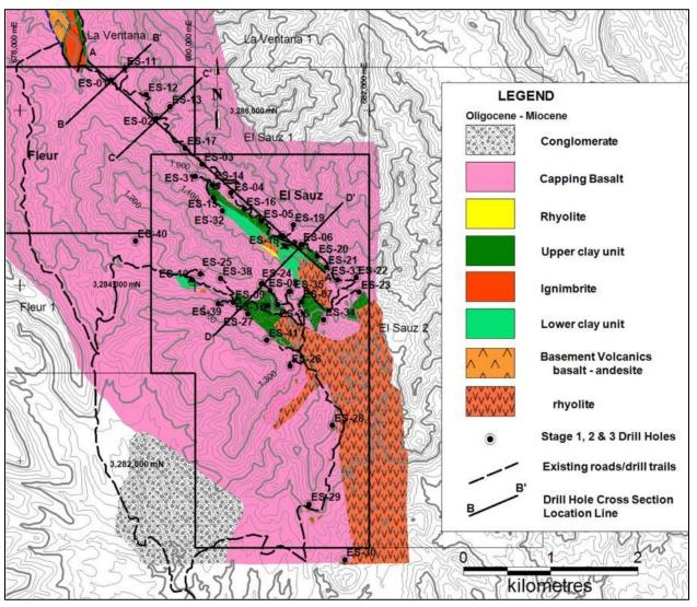
Figure 13. Location Plan of Stage 1, 2 & 3 Drill Holes El Sauz & Fleur Concessions.
