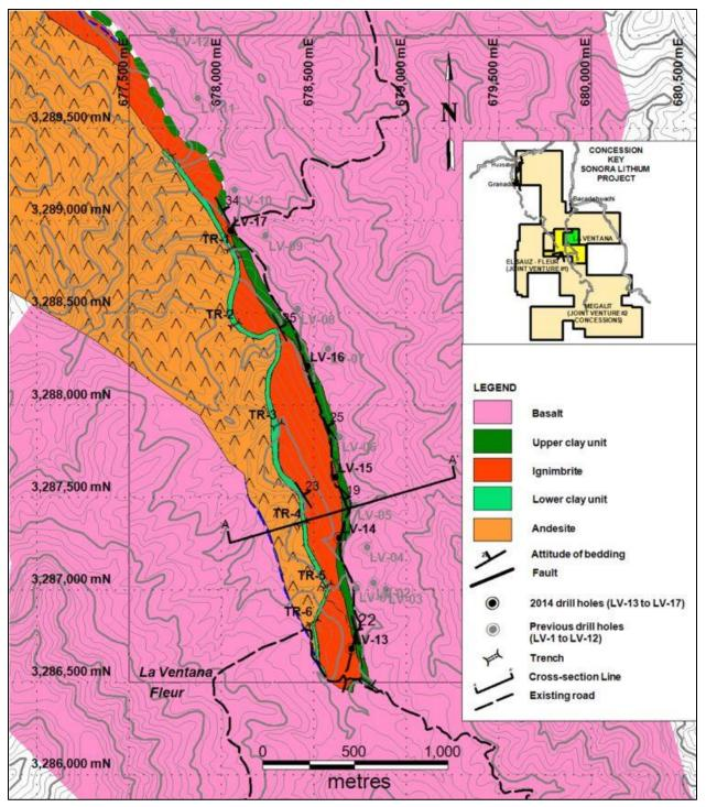
Figure 11. Drill Hole Location Plan La Ventana Concession.
